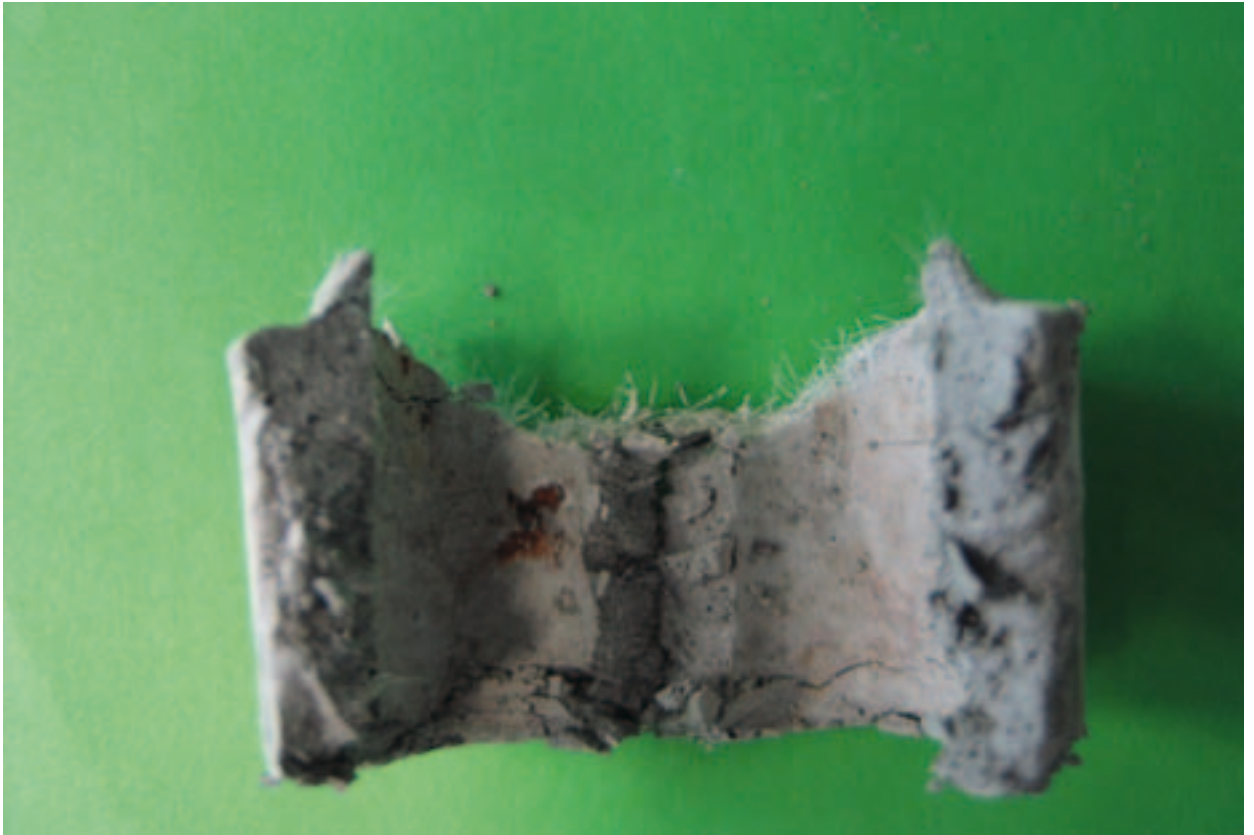
Photo. 4a. Cement stone with fiber and granulated rubber (annular space fragment)
