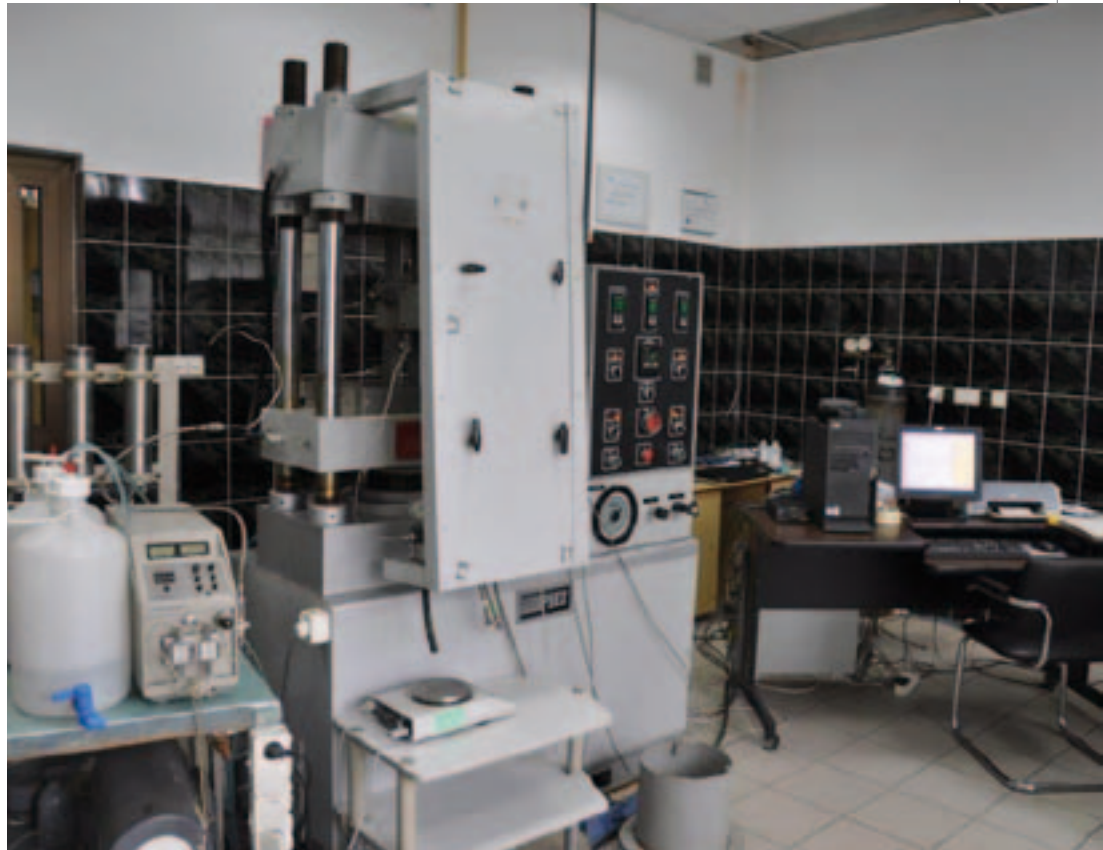
Photo 1. Workstation for proppant conductivity tests (source: KS Plant’s own materials)
