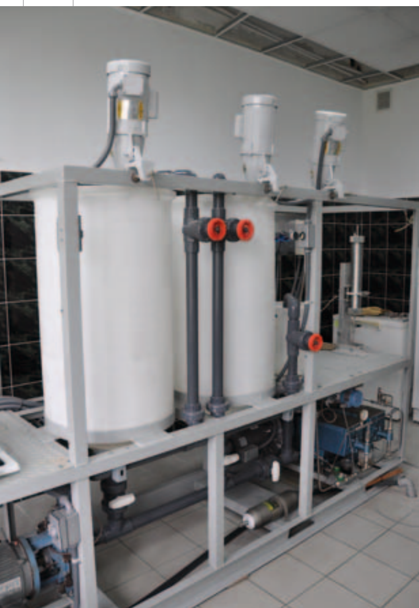
Photo 2. Workstation for rheological examination of fluids for hydraulic fracturing (source: KS Plant's own materials)
