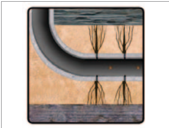
Fig. 14. Diagram of fracturing with the use of solid fuels in horizontal borehole [6]
