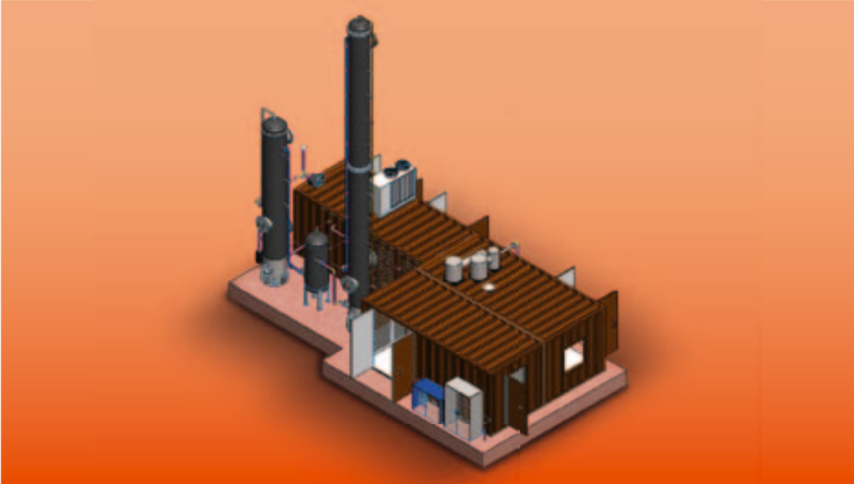
Fig. 4. Installation for biogas to biomethane upgrading
