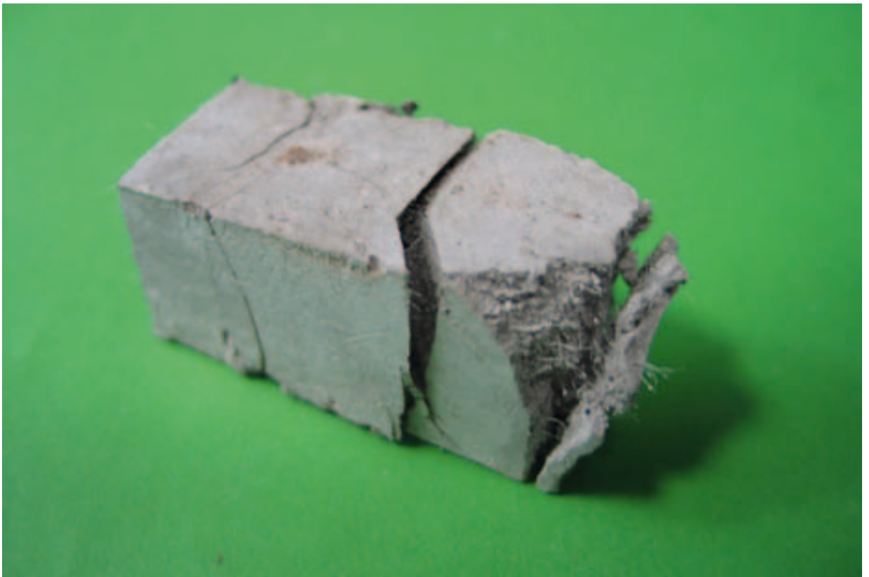
Photo. 4b. Cement stone with fiber and granulated rubber (girder fragment)
