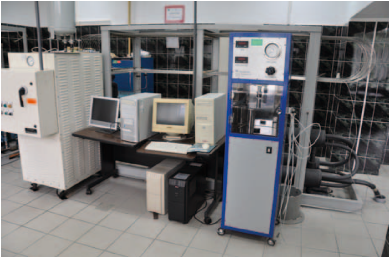
Photo 3. Fragment of research workstation for stimulation of fracturing fluid flow on semicommercial scale (source: KS Plant's own materials)
